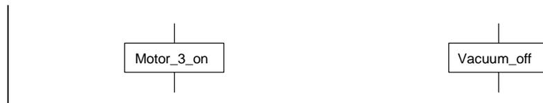
All steps in a program or function block formulated in a sequential function chart must have different names. Even if two steps have the same execution parts, these are to be designated twice.
