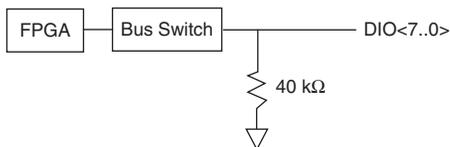
When a DIO line is floating, it floats in the direction of the pull resistor. A DIO line may be floating in any of the following conditions:
