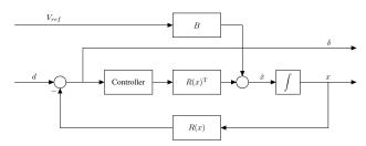
Fig. 2: The formation control is augmented with an additional controller to eliminate the steady-state error in the formation.
