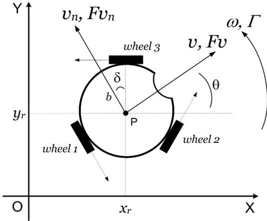
(a) Geometric parameters and reference frames.
